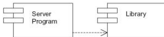
The physical hardware is made up of nodes. Each component belongs on a node. Components are shown as rectangles with two tabs at the upper left.
