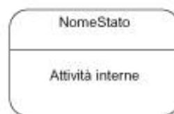
A state is shown as a rectangle with rounded corners. Optionally, it may have an attached name tab. The name tab is a rectangle, usually resting on the outside of the top
